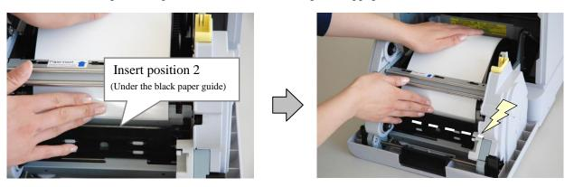
7. Set the take-up side core of the ribbon to the printer. Insert the protrusion of the core left side in the hole on the printer, then set the right side to the holder of the same color (yellow).
