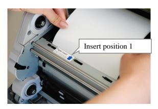
5. Fit the paper to the proper position for each size.
