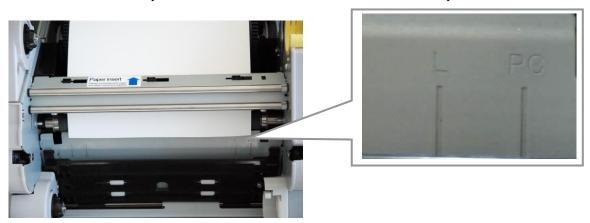
6. Insert the paper under the black paper guide until the buzzer beeps (approx. to the dotted line). Make sure to insert the paper straight. If it isn't inserted straight, the paper will be crooked, which could cause white line on the edges of the print, ribbon wrinkles, and register slippage.
