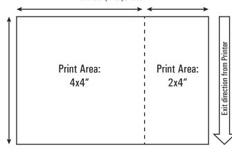
The DS40 printer recognizes media as a standard 4x6 sheet. Layout design is user-defined and needs to accommodate the perforation.
