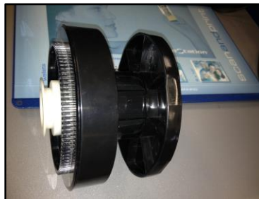
Spacer on paper holder, not pushed all the way into position.
