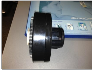
L-spacer installed correctly.
