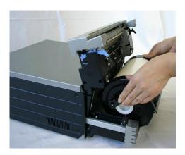
9. Turn the paper in the direction of the arrow. When it is advanced enough, the buzzer will beep, and the flashing LED (orange) will go out.
