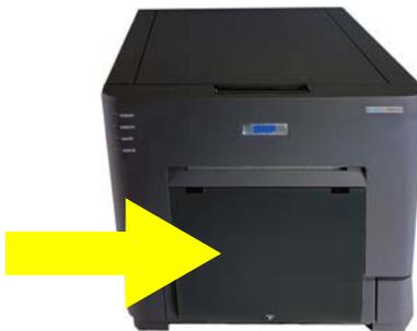
2. Press the release lever on the top of the printer to open the media door.
