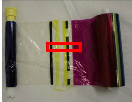
4. Replace the ribbon in the printer and wind the ribbon a few times to remove any slack and until the tape is no longer seen.
