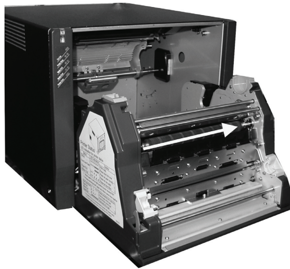
Figure 13. Cleaning the Platen Roller
