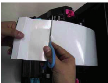
Figure 27. Cutting the Damaged End off the Roll
