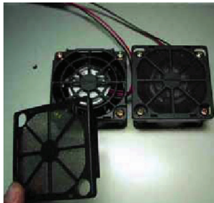
Figure 8. Removing the Fan Filter Cover
