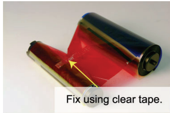
Figure 18. Fixing a Torn Ribbon
