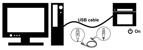
Connect the USB cable, switch on the printer, and then install the printer driver.
