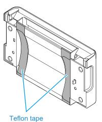
3 Attach the printer unit's trash box.
