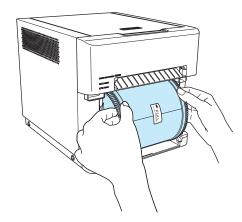
9 Remove the seal, place a hand on the paper, and rotate the paper holder in the direction of the arrow to insert the paper leading edge until the buzzer beeps.
