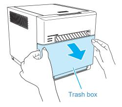
2 Dispose of paper scraps. (Several sheets of paper scraps may remain in the trash box.)
