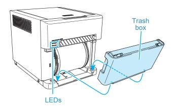
Printing is not possible with the trash box removed.
