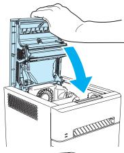
5 Remove the printer unit's trash box.
