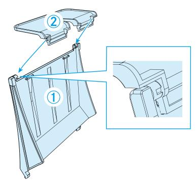
2 Insert and push the pegs into the hooks.
