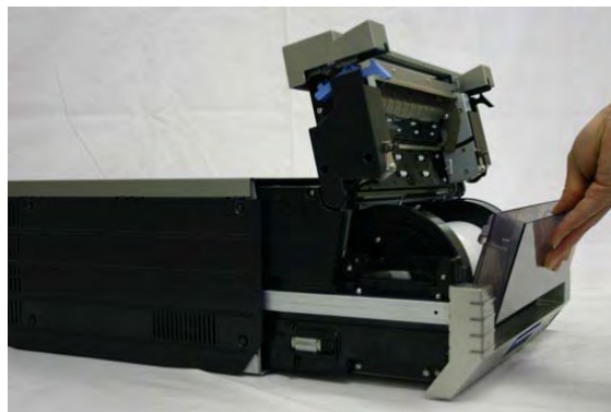
Figure 34. Removing the Scrap Bin
