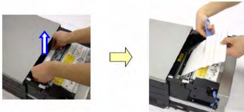
Figure 40. Pulling and Trimming the Paper
