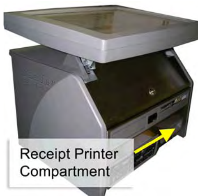
Figure 1. Accessing the Receipt Printer Compartment
