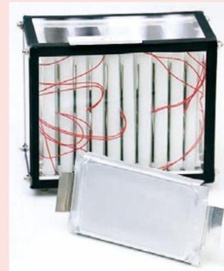
These pouches can be easily configured for specific applications and are now widely used as a primary component in electric and plug-in hybrid vehicles.
