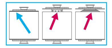
2. **Mount the paper roll onto the paper spools.** Locate your new printer media and remove one paper roll and one ribbon. Make sure the paper roll is oriented so that the leading edge of the paper roll is coming over the top of the paper roll and directed towards the front and bottom of the paper roll.
