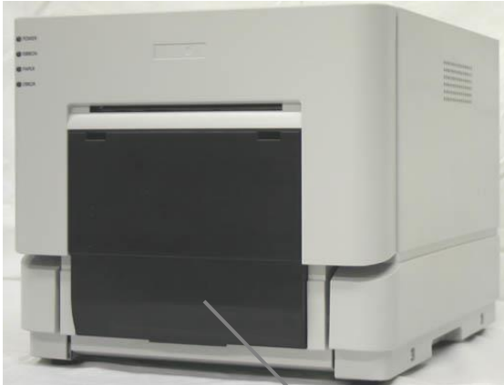
Printer Unit Scrap Box
