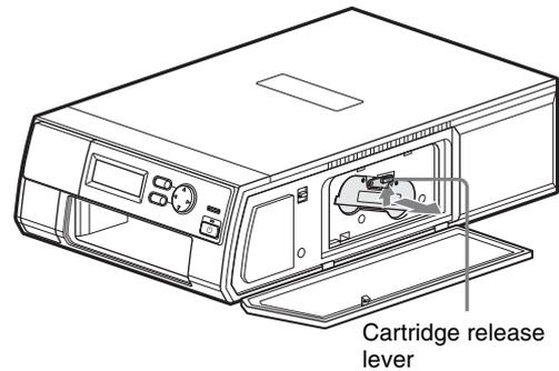
Remove the print cartridge when it ejects.
