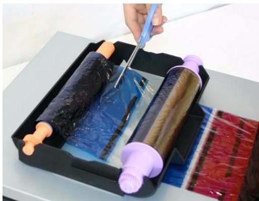
Figure 9. Cutting the ribbon
