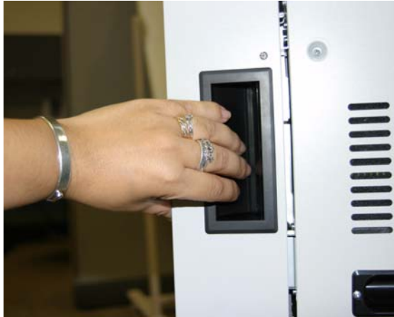
Figure 1. Opening the Tower Door
