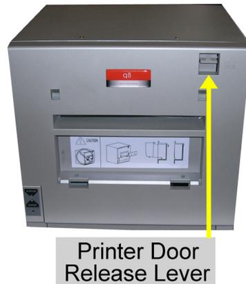
Figure 38. Door Release Lever
