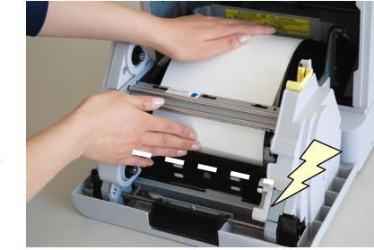
5. Remove a paper fixed tape, and insert the paper.
